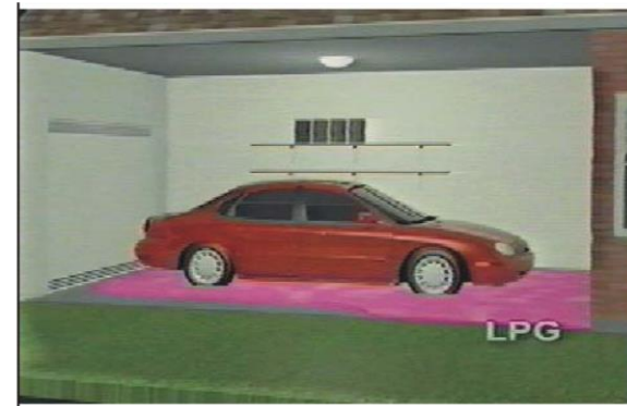
Liquid Propane Leak
