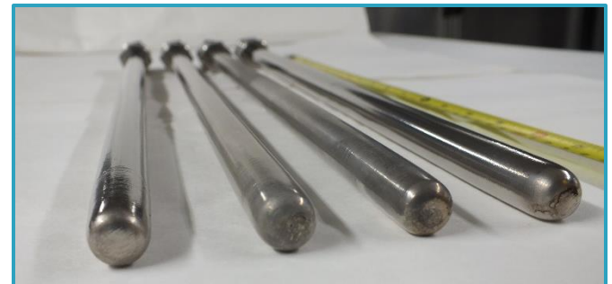
2 nd generation thin film Pd-alloy supported membranes (>40 cm long)
